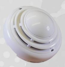
The ZC920 is a 58°C rate compensated RoR heat detector for use in areas where smoke detection would be likely to produce false alarms, for example kitchens and shower rooms. The detector has been certified in Europe to be complaint with the Class A1 requirements of EN54-5 standards. The detector uses a thermistor to detect heat and rate of rise algorithms for alarm trigger from any temperature starting at -10°C to its static trigger point of 58°C.
